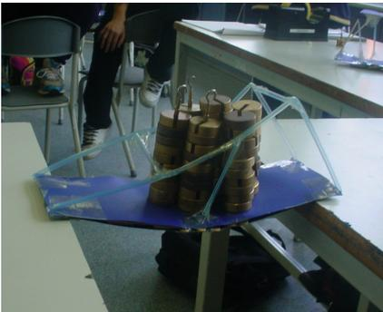
*"Some ideas we used were to make our bridge longer than the 25 cm gap. We tried to build a beam/truss bridge with a very strong deck, the deck worked, but the beams on the sides did little more than hold the weights in place."*
