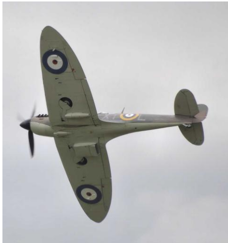
A Supermarine Spitfire from below, showing the elliptical wing design that minimises drag. (Image from http://upload.wikimedia.org/wikipedia/commons/8/8b/Spitfire_mk2a_p7350_arp.jpg )
